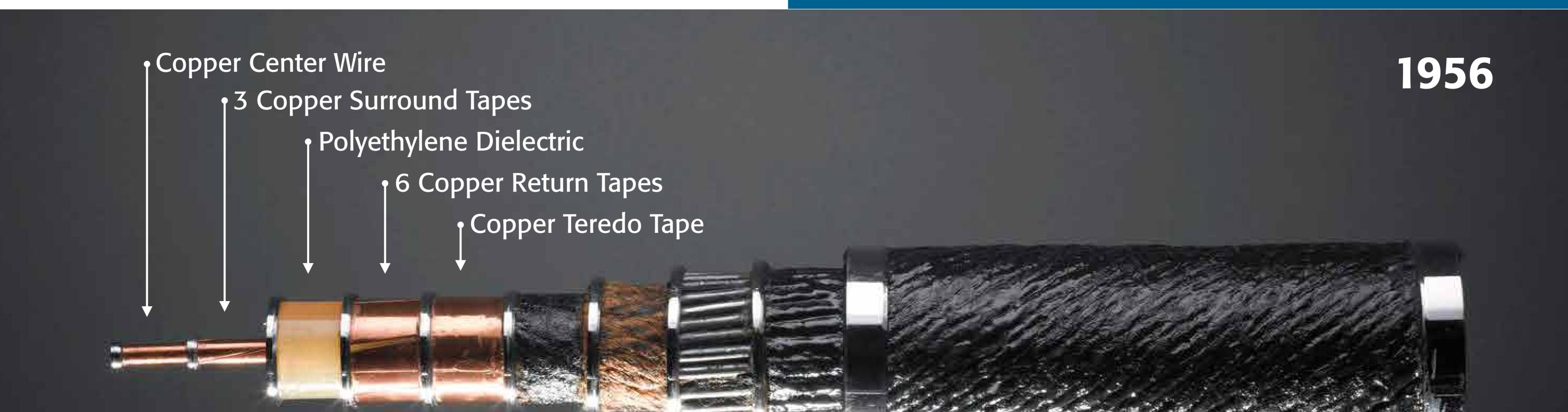
Treated Cotton Tape Jute Bedding with Binding String 24 Cotton-Covered Armor Wires
