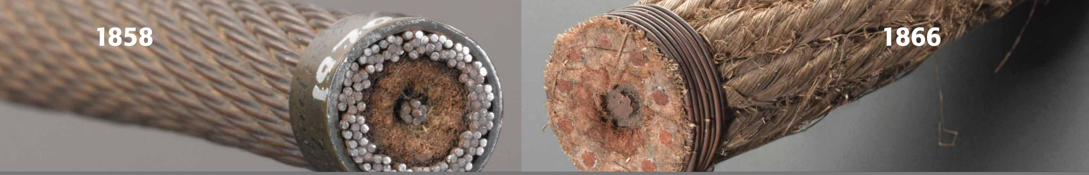
The failure of the first transatlantic telegraph cable, laid in 1858 (above left), was blamed partly on a lack of electrical standards and testing procedures, particularly for resistance. This was put right for the successful cable of 1866 (above right). It consisted of seven strands of gutta-percha insulated copper wire, and was protected by
