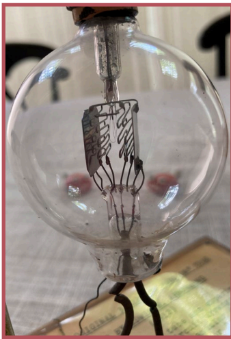
The two-filament, two-grids, and two-plate Audion tube owned by Howard Armstrong
